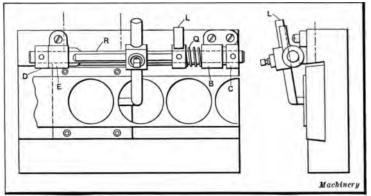
Fig. 37. The Side Swing Latch Stop
